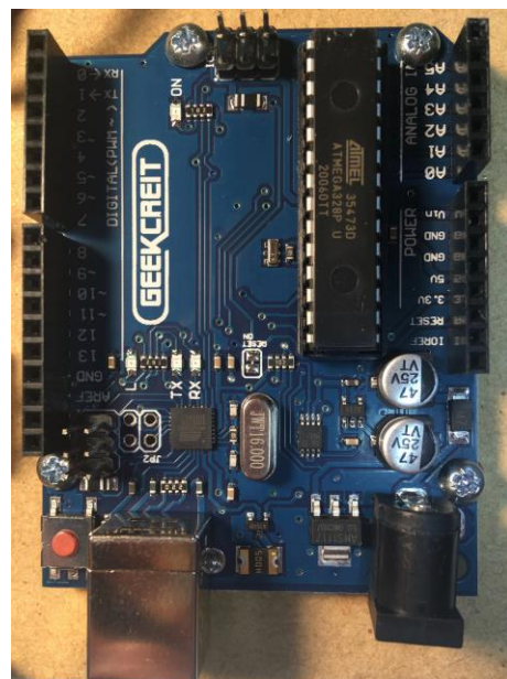
USB Lead to PC Socket for 12vdc Plug (optional) Arduino UNO
